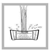
3. Rinse the sample cup with the sample. Make sure to use a filter to remove particulates from wastewater and effluent samples before analysis.
