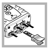
2. Put the Chemkey quickly in one movement into any slot. Carefully remove the packaging from the Chemkey.
