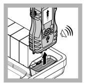
6. Wait for the sound alert and/or the meter removal animation (within 1 to 2 seconds), then immediately remove the meter from the sample cup.
