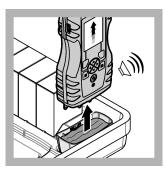
**6.** Wait for the sound alert and/or the meter removal animation (within 1 to 2 seconds), then immediately remove the meter from the sample cup.
