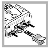
2. Put the Chemkey quickly in one movement into any slot. Carefully remove the packaging from the Chemkey.
