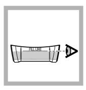
**4.** Fill the sample cup to the fill-line with sample.
