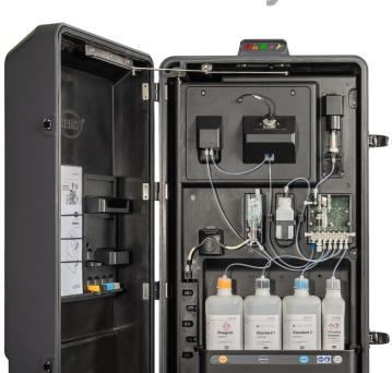
Simplify your online operations with the NH6000sc, an online Ammonia Analyzer using gas sensing electrode (GSE) technology. The environmentally controlled design is ready for easy, outdoor installations at the measurement point you need. With minimal maintenance requirements and proven reliability, Hach's NH6000sc will give you confidence in your measurement results and improved process efficiency.
